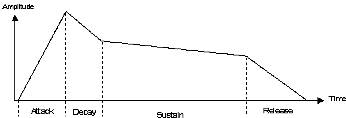
Figure 3: Parameters of a note. Courtesy of MIDI Manufactures Association – Used with permission.
